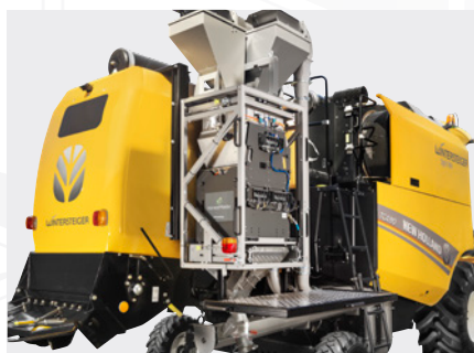
Powerful weighing system Twin H2 from HarvestMaster, with precise weighing, moisture and volume weight data
